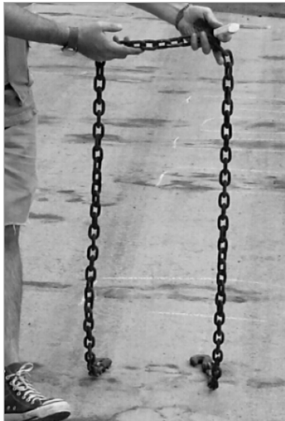
Figure 8.7 Chain drag test to detect delamination
